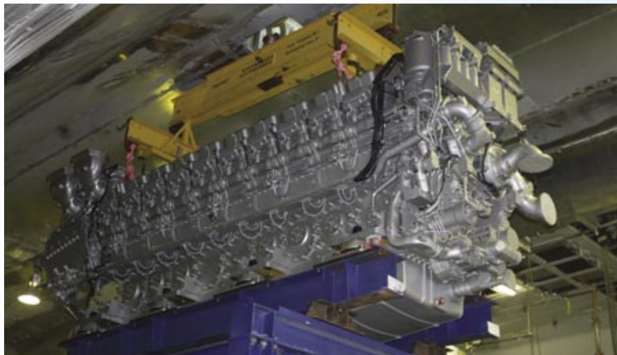
• The MTU 8000 Series diesel engine ready to installation.
