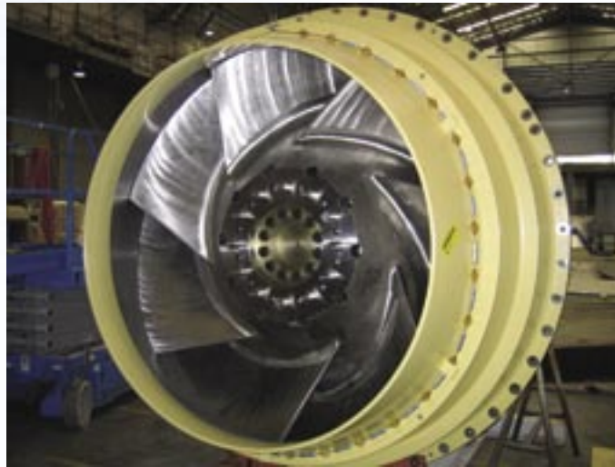
• The 180 BII 7B Kamewa central booster jet while still in the factory at Rolls-Royce AB.
