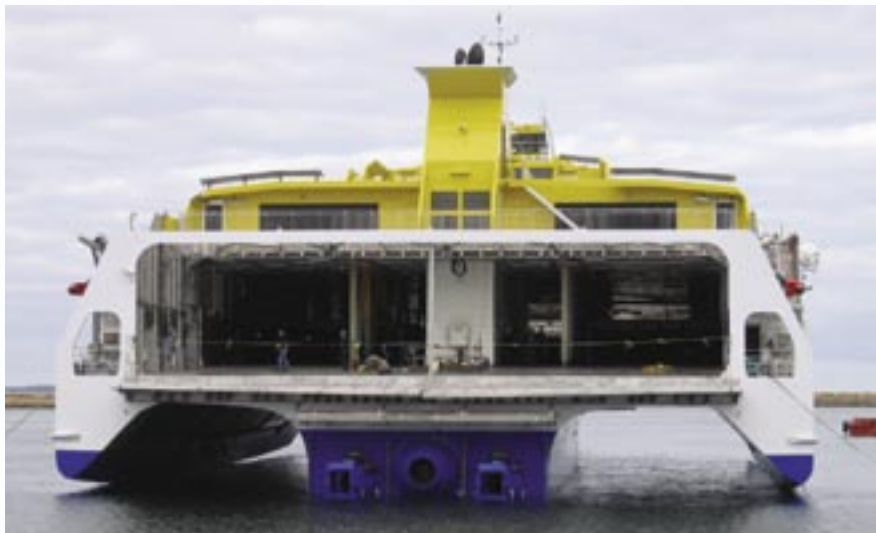
• "Benchijigua Express" a launch day showing stern and waterjet arrangement
