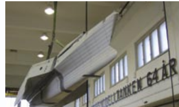
• 5 metre tank test model used for seakeeping analysis.
