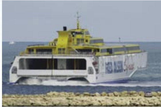
• Transom design enables full beam car and truck loading and unloading.
